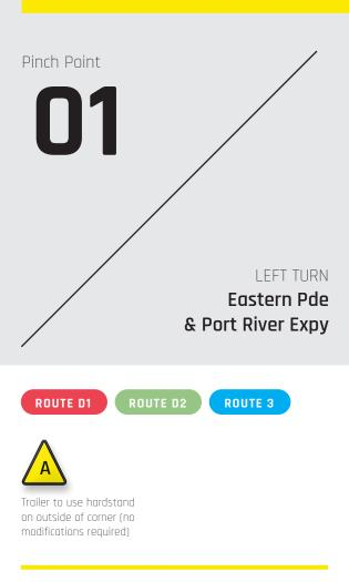
This corner was taken by Ares for similar blades for the Silverton project with no issues. The blade trailer will need to track off the asphalt on the outside of the corner in order to avoid the traffic lights on Eastern Parade. This area is generally suitable, with the option to add hardstand material to it if required for added stability.
