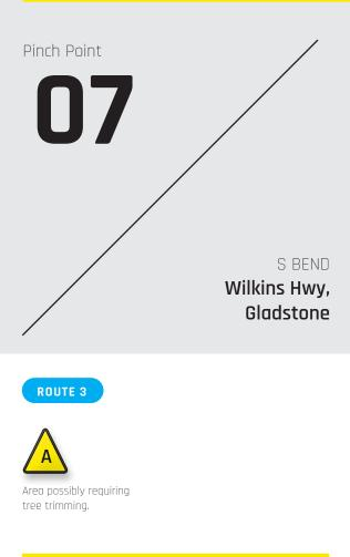
The compound S-bend in Gladstone can be taken with no modifications, but will require traffic to be held at both ends while the blade trailer is traversing this section of road. Some tree trimming may be required to accommodate the blade swept path.
