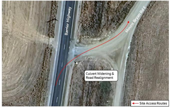
Figure 6 2: Barrier Highway / White Hill Road realignment. Credit: Google Earth 2023
